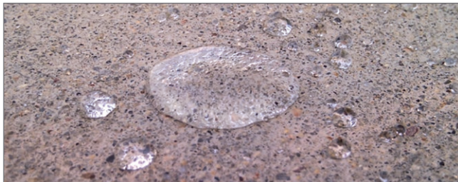
Photo demonstrating the ability of DuraSeal to repel water with its hydrophobic barrier.
