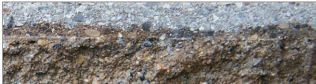
Cured with DuraCure and sealed with DuraSeal . Dry area demonstrates the depth of sealer.
